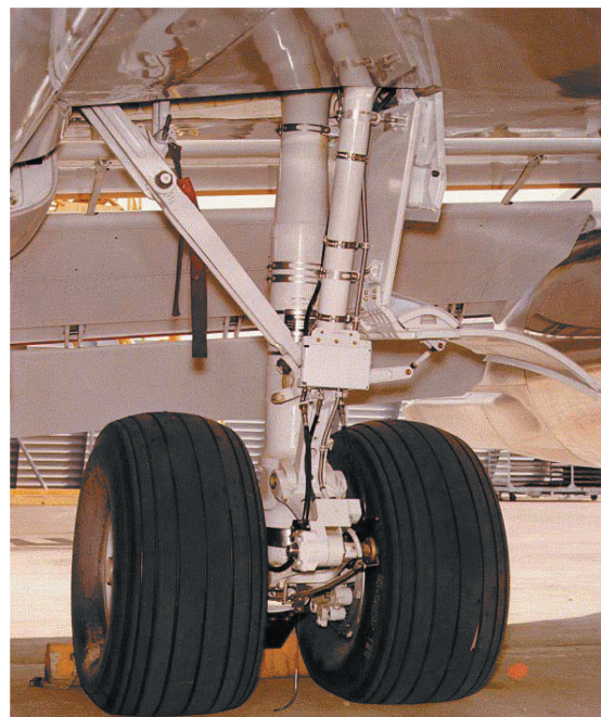
Fig. 4 Full-scale Boeing 737 main landing gear.
